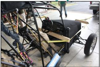
One of the required ASTM tests was confirming the integrity of the seat frames and harness. The Maverick was stretched between the forklift and the Diesel Truck.
