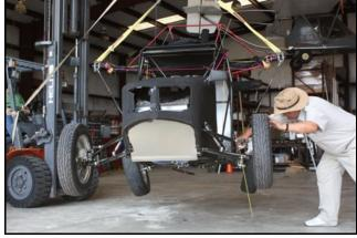
Sandbags were added to make the chassis weigh beyond its allowable gross weight. Then the Maverick was raised above our cement floor and the rope was cut. After dropping, the Maverick was examined for structural failure. (The Maverick passed the test with flying colors)
