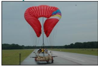
Another FAA requirement was to take our parachute "wing" up to cruising speeds, purposefully collapse it, and document its recovery process. To perform this test, we loaded the trailer with 6,000 lbs of ballast sandbags to keep it on the ground.
